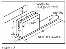
Make three corner-holders as shown in Figure 2. These will establish the reference plane as parallel to and offset 3" from your work surface. The tongue extensions provide places for weights to keep the holders in place while measuring. Make a pair of straight-edge holders as shown in Figure 3. These holders will allow a straight-edge to be held over the sail, perpendicular to the luff, and just touching the luff and leech, representing the chord of the sail at that height.
