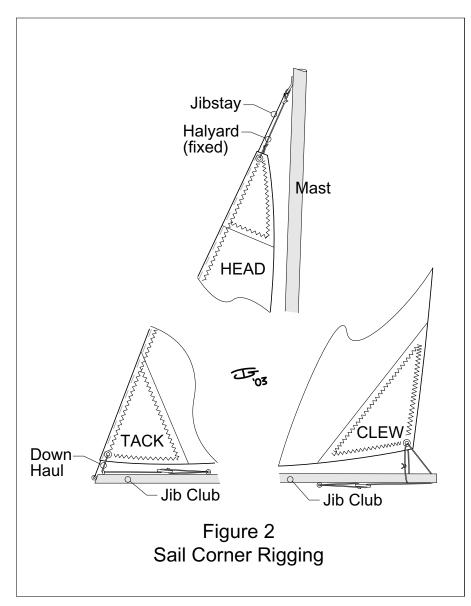
and makes for a smooth and clean entry where the wind meets the sail. The luff hem method eliminates scalloping which can happen with the tubes, and it distributes the wind load evenly over the entire luff. Some jibs are mounted using little hollow tubes affixed to the sail that are slid over the jibstay. The sail tubes provide for excellent swiveling as the sail tacks, but produce point loads where they attach to the sail, and this can cause the sail to wear out prematurely.
