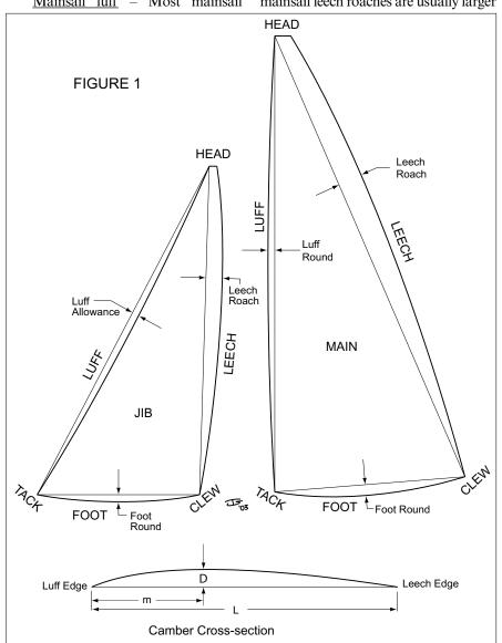
than jib leech roaches. Care must be taken that the battens are not so stiff that they flatten the after third of the sail to look like a barn door. Battens on modern sails assist in shaping the after parts of the sail, the cloth is generally stable enough to hold itself fairly well, needing just a bit of help.
