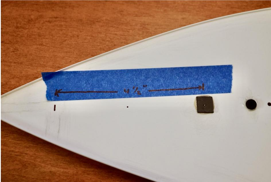
I moved the little screw that is used for the jib boom hold down bowsie back to 4 1/2" (11.5cm) from the jib hold-down loop to allow for more adjustment. Again, back up with a small piece of thin plastic or carbon fiber plate.
