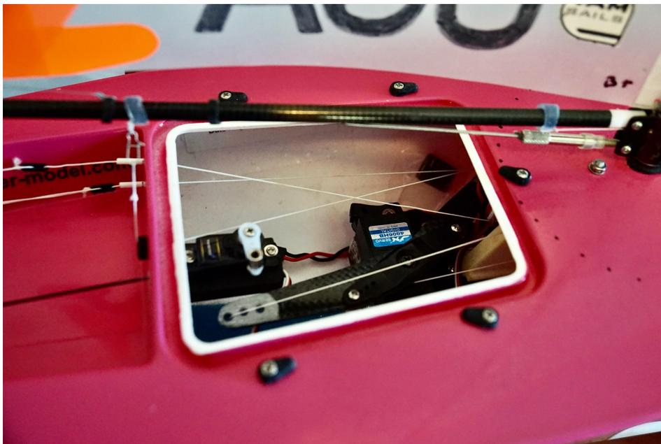
The threading of the main sheet adjuster is easy. For the jib sheet adjuster, pass the sheet through the little tube adjacent to the sail servo board and then around the front of the keelbox to the swingarm.
