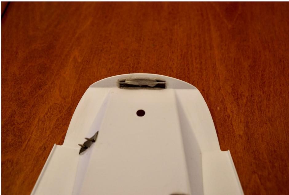
Instead of using the Hacker hull backstay fitting, I simply used a cotter pin backed with a small piece of this carbon fiber plate. (Some ABS or other thin plastic would work fine as well.) Hold the cotter pin in place with some small clamps while it is drying.
