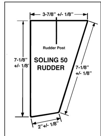
**RUDDER:** Construction materials are optional. (See Soling 50 Class Rules - 2009)
